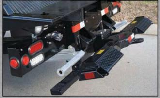
LED body lighting, anti-theft L-arm storage, easy access safety chains and a trailer hitch adapter are just a few of the many standard features that have been designed into the Champion carrier to provide for ease of operation.
